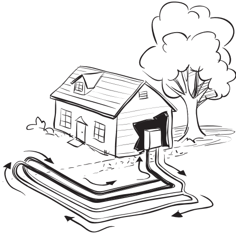
Geothermal Heat Pump
